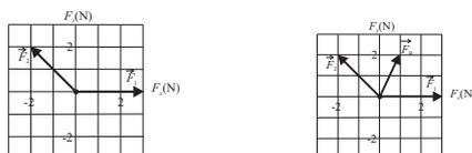
$$a_x = \frac{F_{R,x}}{m} = \frac{1 \text{ N}}{2 \text{ kg}} = 0.5 \text{ m/s}^2$$
